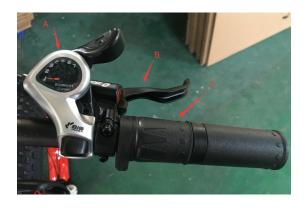
A: Shimano 7/9 Speeds Rear Gears Lever;
