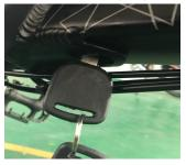
When battery key cylinder pulls back fully and then take off the key
