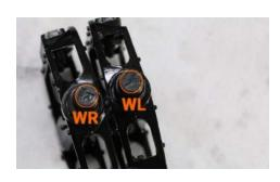
WR/R is for Right Crank; WL/L is for Left Crank;
