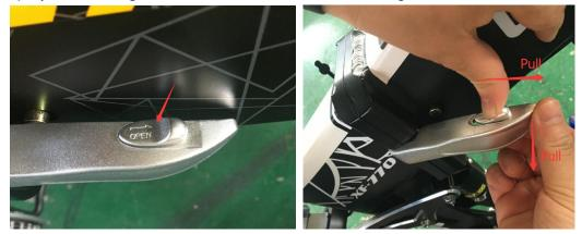
1) Open the folding frame locker . Find the latch on the folding frame locker.
