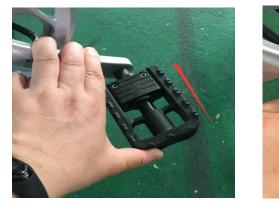
Push and press pedal inward and then fold the pedal
